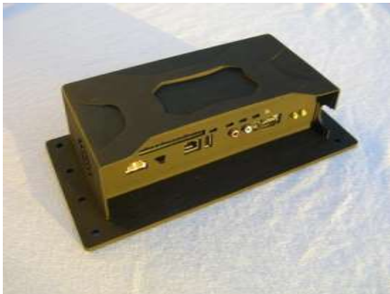
Figure 4. Picture of the main DAS unit, installed in the rear of the vehicle.
