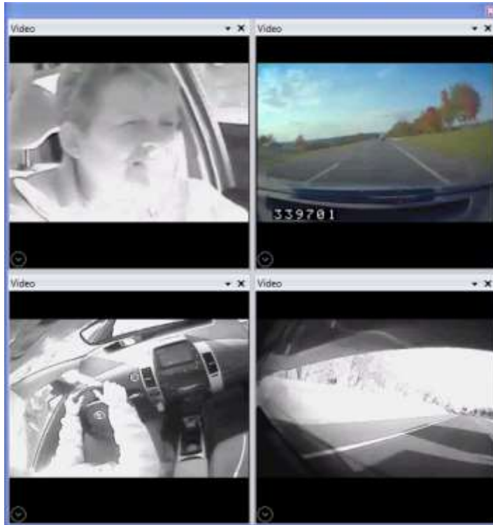
Figure 5. Quad image of driver (VTTI employee) face (upper left), colour forward view (upper right), over-the-shoulder (lower left), and rear view (lower right).
